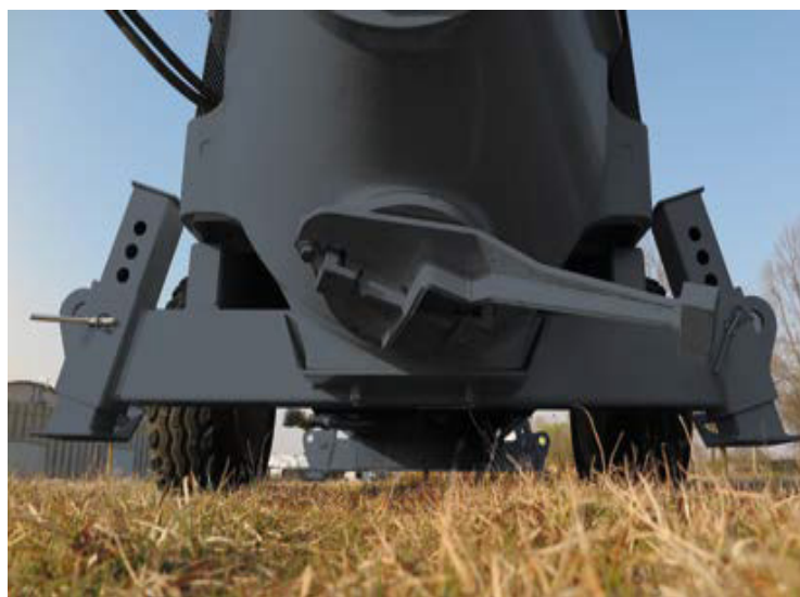
Unloading door for optimal cleaning of the hopper.
