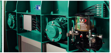
Automatic lubrication system equipped with 4 programmable and independent pumps
